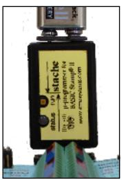
When you connect the Stache to a good 9 volt battery, the green light will flash briefly. Plug the Stache into the programming connector on your Stamp project or carrier board. Refer to the box if you do not have a standard connector and need to construct an adapter. Be sure the power to your project is also turned on—the Stache battery does not power your Stamp
